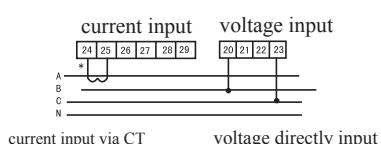
current input via CT      voltage directly input
