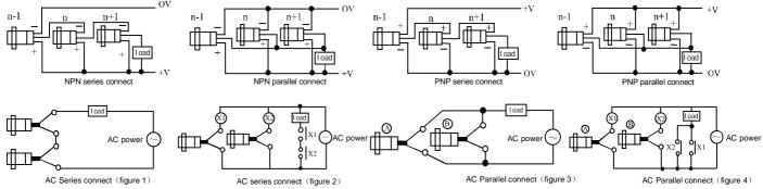
If the power supply is 220V, and the quantity of connected sensor is less than 3 ,connect as figure 1 ,otherwise
