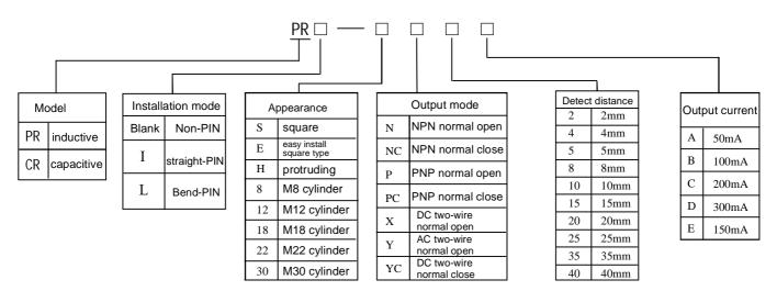
For example: PRI-12N4C means straight -PIN connecting, DC inductive proximity sensor, diameter 12mm, NPN normal open, detecting distance 4mm, Max. output current is 200mA
